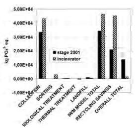
Fig. 9. Eutrophication caused by two Krakow MSWM systems
