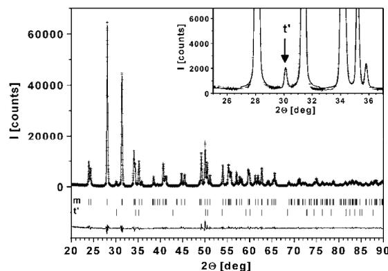
Fig. 1. Rietveld refinement plot of the annealed ZrO<sub>2</sub>:Pr. The inset documents the presence of 101 reflection of tetragonal phase.
