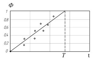
Fig. 4. Determination of the diffusion coefficient D
