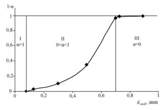
Fig. 5. The influence of the size of the raw material grinding on the degree of extraction of oil, in the form of dependence  $1-\alpha=f(d_{mid})$
