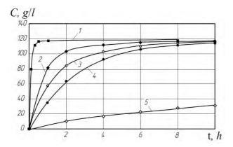
Fig. 1. Kinetics of oil extraction for not grinded and grinded sunflower seeds of different fractions with n-hexane at the boiling temperature of the solvent in the apparatus with a mixer: 1 – grinded seeds with  $d_{midl} = 0.3$  mm; 2 – grinded seeds with  $d_{midl} = 0.5$  mm; 3 – grinded seeds with  $d_{midl} = 0.75$  mm; 4 – grinded seeds with  $d_{midl} = 1.25$  mm; 5 – not grinded seeds
