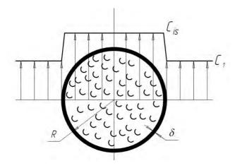
Fig. 3. Scheme of a simplified physical model of extraction of target components from sunflowers eeds ( $\delta$  – film thickness,  $C_1$  – the concentration of oil in the main mass of solution,  $kg/m^3$ ;  $C_{is}$  – the initial concentration of oil in the seed,  $kg/m^3$ )
