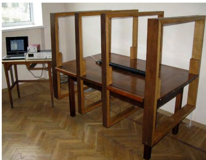
Fig. 3. Laboratory installation for analysis the Helmholtz coils using the multifunctional gain-phase analyzer
