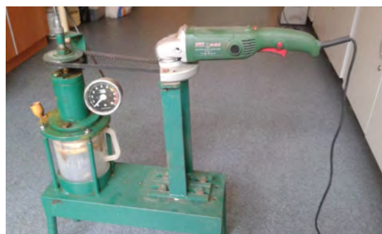
Fig. 1. Setup for studying hydrodynamic cavitation in the process of adsorbent obtaining
