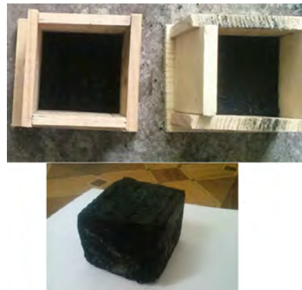
Fig. 4. Forming of samples of masonry units
