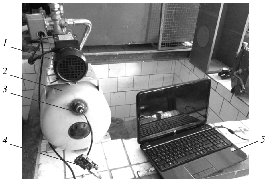
Fig. 2. Experimental setup for the study of transient gas processes in the bladder-type hydraulic accumulator: 1 – pump PKM60; 2 – hydraulic accumulator with a nominal volume of 24 \text{ dm}^3 ; 3 – DC pressure transducer; 4 – controller based on Arduino UNO R3 board; 5 – computer
