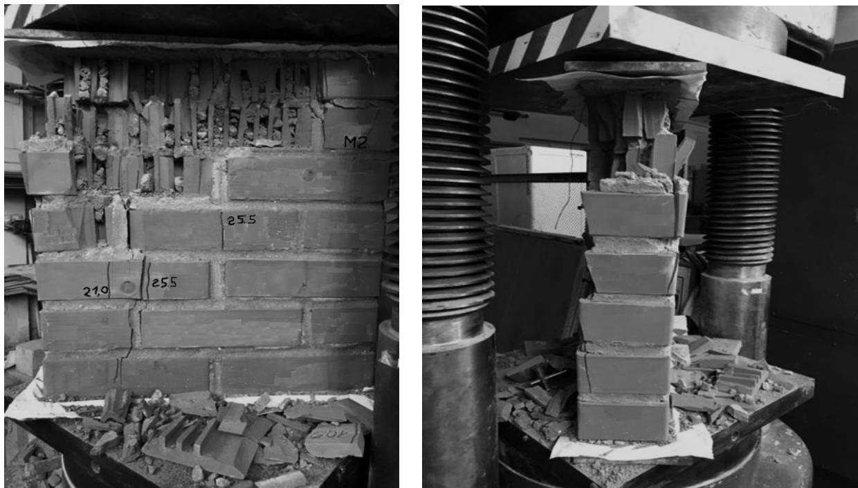
Fig. 1. Determination of compressive strength of masonry
