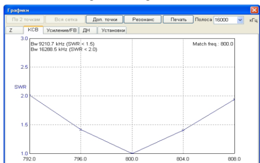
Fig. 8. A amplitude-frequency response (AFR) of unloopback vibrators 10×10 (bandwidth reached 2%), synthesized by means of ACO algorithm (fig. 2.a).
