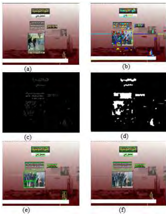
Fig. 2. Text detection : (a) original image , (b) MSER extraction in image (a) , (c) Image mask integrating MSERs and canny edges (d) open result , (e) candidate text regions , (f) final result.
