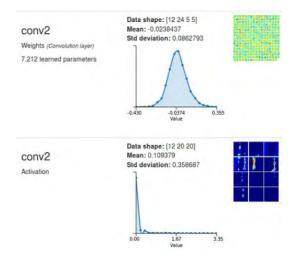
Fig. 6. Image processing on the second convolutional layer
