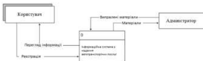
Fig. 4. The context diagram of the information system of ordering motor transport services
