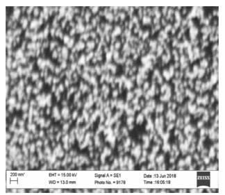
Fig.1. SEM images of n-Si (100) surfaces of silicon with gold deposited by galvanic replacment in DMSO solutions at the temperature 40 °C
