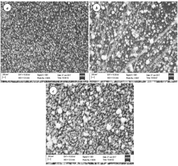
Fig.2. SEM - images of gold nanoparticles deposited from a solution of 4 mM HAuCl<sub>4</sub> in DMSO on a silicon surface for 1 min at a temperature of 50 (a), 60 (b), 70 (c)  $^{\circ}$ C
