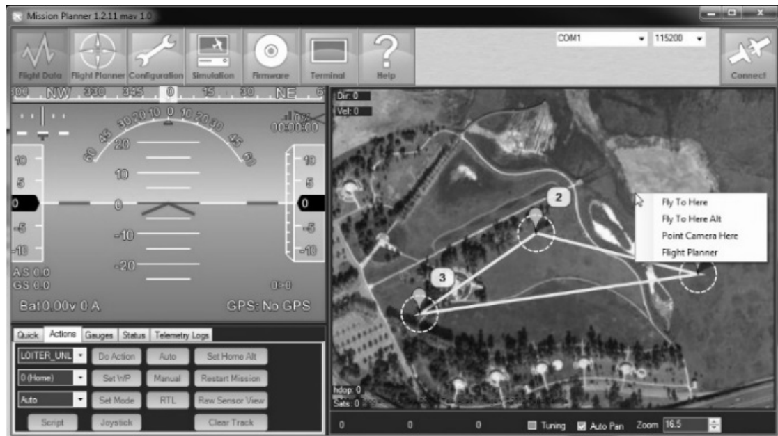
Fig. 4. Receiving telemetric data by the Mission Planner program, fixed by the projected ornithopter.
