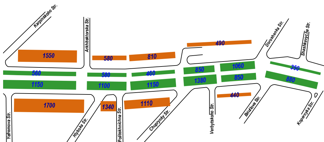
Fig. 2. Section of S. Bandera street indicating hourly traffic and pedestrian flow on its segments [14]
