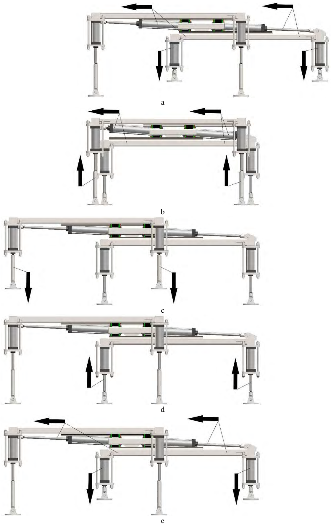
Fig. 2. Graphical interpretation of the main motion cycles of mobile robotic system with orthogonal walking drive
