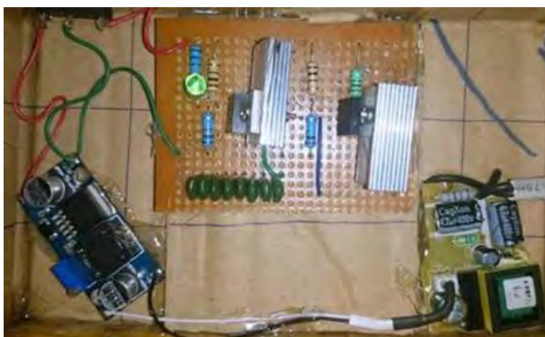
Fig. 11. Components on the Veroboard.
