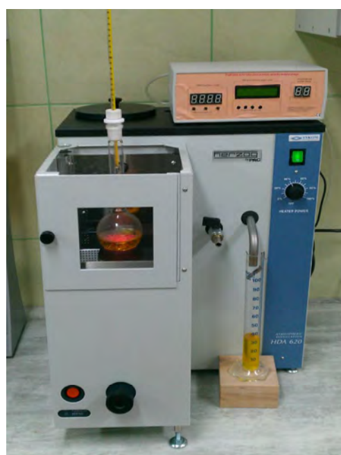
Fig. 3. Photo bench equipped with a distiller HAD 620/1 by Herzog
