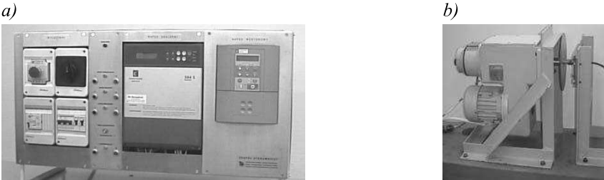
Fig.7. Training device for testing and tuning PLC controlled drives: a) set of three devices for supplying asynchronous motors (relay-contactor circuit and two different inverters), b) example driving unit with asynchronous motor, gear box switched by means of electromagnetic friction clutches and encoder for closed loop positioning
