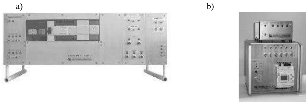
Fig. 1. Training stand for testing PLC application programs: a) device with Mitsubishi FX2N PLC controller and with additional replaceable function modules, b) device with Mitsubishi Alpha controller
