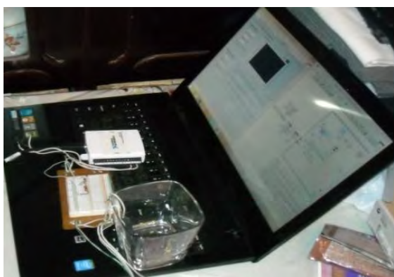
Figure 6. Virtual device for measuring the contamination of the heavy metals in the juice
