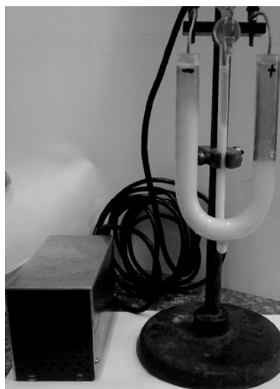
Fig. 2. Electrophoresis of Ca(OH) 2 suspension with Burton’s apparatus
