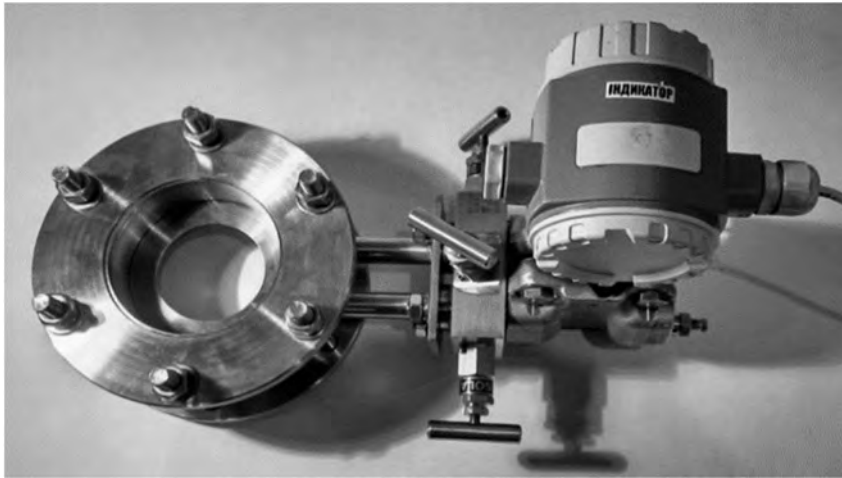
Fig. 6. General view of the flow meter for measuring the compressed air flow-rate in the pipeline downstream of the multi-compressor system receiver.
