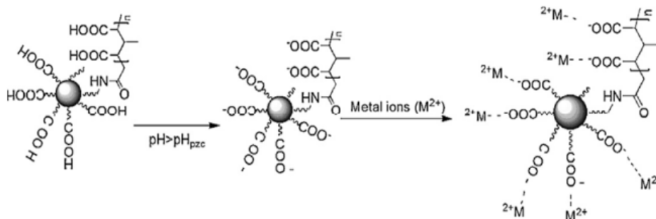
Fig. 13. Schematic representations of possible mechanism for adsorption of metal ions by \text{Fe}_3\text{O}_4 @APS@AA-co-CA [1]
