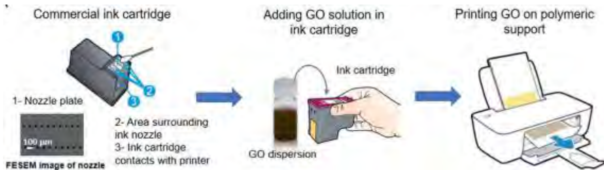
Fig. 9. Printed, ultrathin grapheneoxide (GO) membranes:
