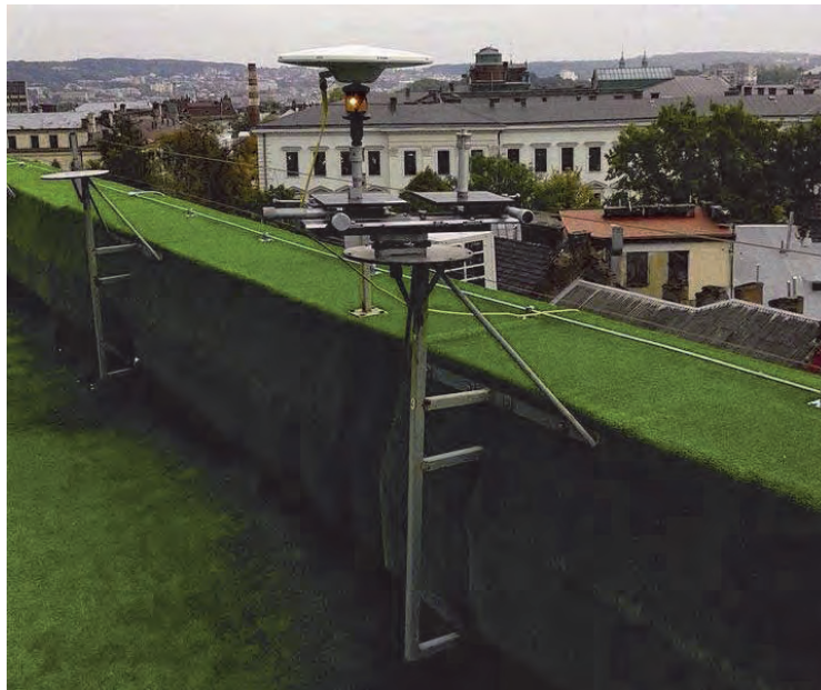
Fig. 3. Device for deformations simulation at the station DAH2
