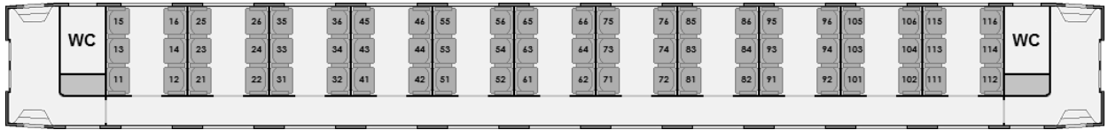
Fig. 2. Schematic of the seating arrangement in a rail car with a coupe [5]
