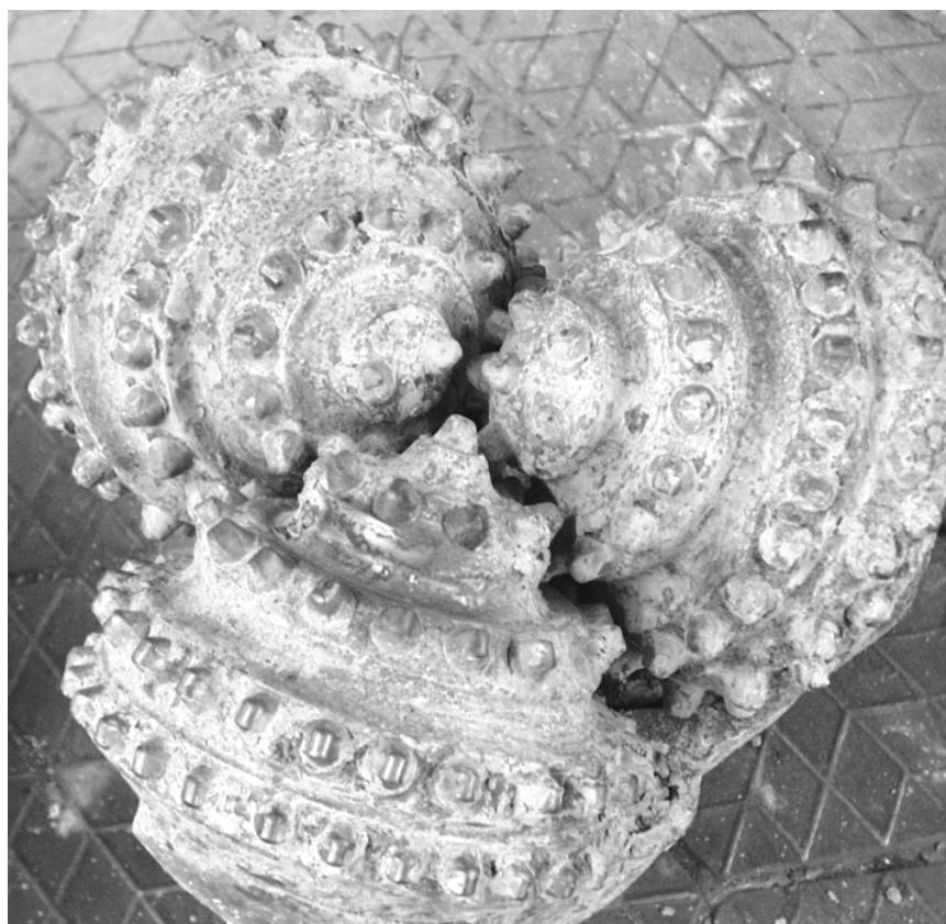
Fig. 1. Appearance of the destroyed roller three-cone drill bit
