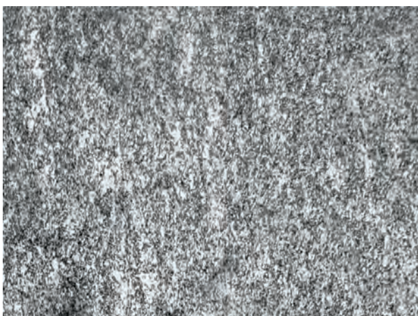
Fig. 4. Microstructure of parent metal (DOMEX steel 700 ( \times 300 ))
