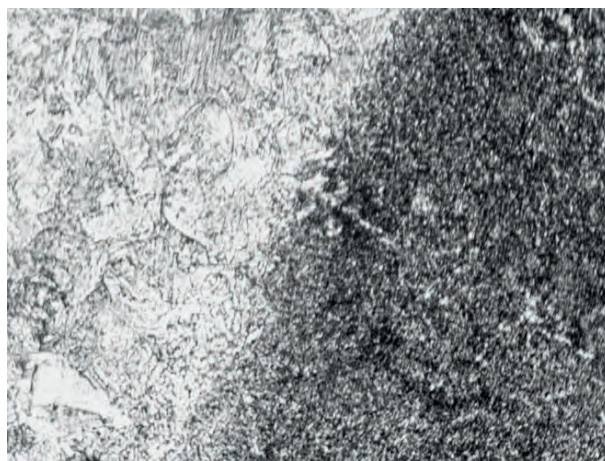
Fig. 7. Microstructure of the fusion zone (x 300)
