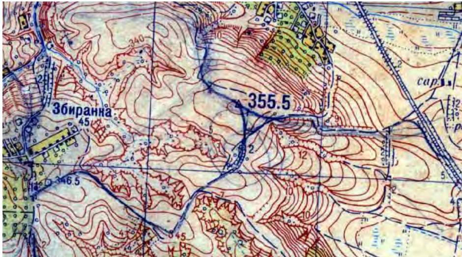
Fig. 1. A fragment of a topographic map scaled at 1: 25 000 with a contour interval 5 m (1957)
