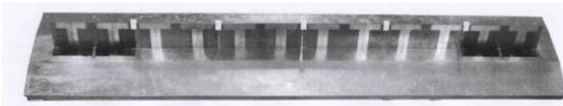
Fig. 8. An experimental sample of an array fragment with microstrip radiators.
