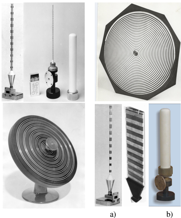
Fig. 1. Modulated impedance surface waves antennas centimeter (a) [6] and millimeter-wave bands (b).
