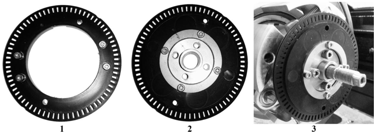
Fig. 2. Design of the sensor for measurement of the rotation angle in a sensitive element of rotational consistency meter [7]: 1 – disk with holes installed on the main shaft of the device; 2 – disk with holes installed on the sensitive element shaft; 3 – optical sensor to determine the sensitive element rotation angle in a paper pulp consistency meter (without opto-isolators)
