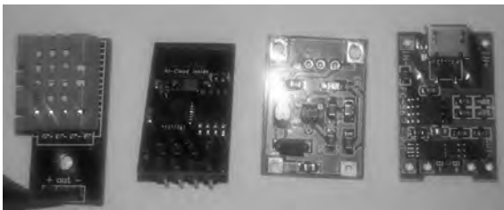
Fig. 8. Components of the prototype of the sensor node
