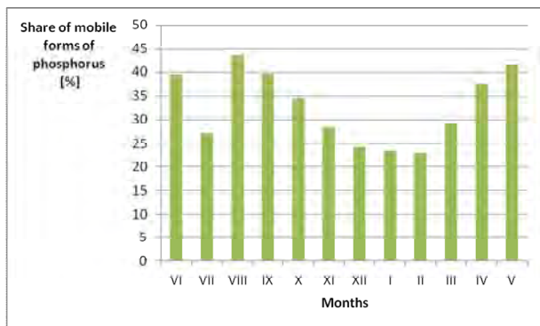
Fig. 4. Share of mobile phosphorus fractions (Ca-EDTA + Na-EDTA) in primary sludge collected at treatment plant B
