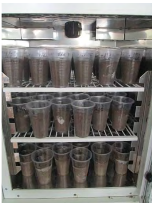
Fig. 1. Storage of samples in the system “soil – fertilizer” ( t = 21\text{ }^{\circ}\text{C} , air humidity – 90 %)
