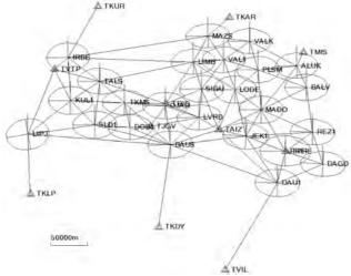
Fig. 2. Adjusted GNSS vector scheme
