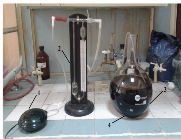
Fig. 1. Photo of the experimental setup: 1 – compressor, 2 – rheometer, 3 – flask, 4 – aerators
