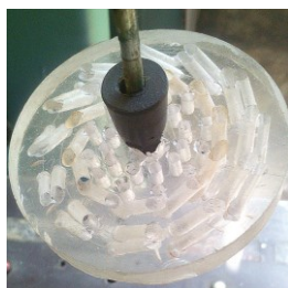
Fig. 6. Swirl generator № 2 – With perpendicular holes in the center and inclined holes along the periphery
