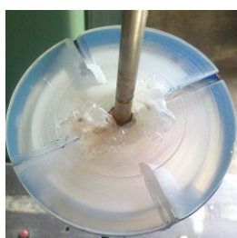
Fig. 8. Swirl generator № 4 – With four inclined slits
