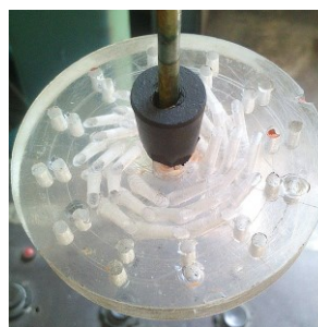
Fig. 5. Swirl generator №1 – With inclined holes in the center and perpendicular holes along the periphery
