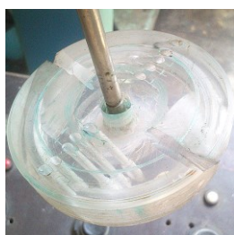
Fig. 7. Swirl generator № 3 – With two rows of inclined holes and two inclined slits
