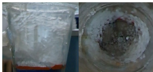
Fig. 4. №4 - The vortex fluidized bed regime with carryover
