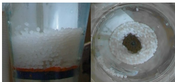
Fig. 3. №3 - The vortex fluidized bed regime
