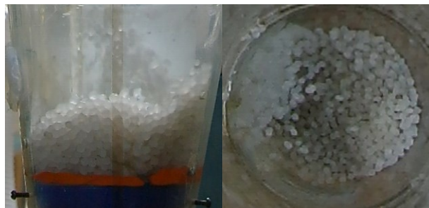
Fig. 2. №2 - The partially fluidized bed regime
