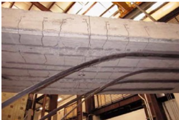
Fig. 2. Illustrations of FRP debonding limit state: debonding at interface between FRP reinforcement and concrete
