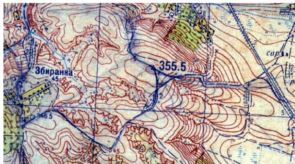
Fig. 1. A fragment of a topographic map of scale 1: 25000 with contour lines of 5 m (1957).
