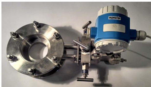
Fig. 3. General view of the measuring unit of the flowmeter of the pulsed compressed air flows, which is executed as a single-welded structure.
