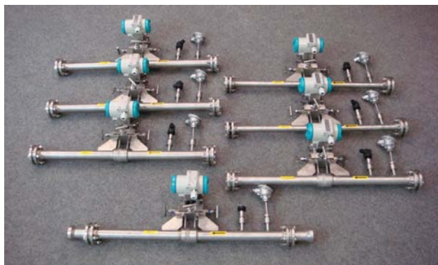
Fig. 2. General view of measuring units of flow meters of pulsed fluxes, executed as a single-welded structure.
