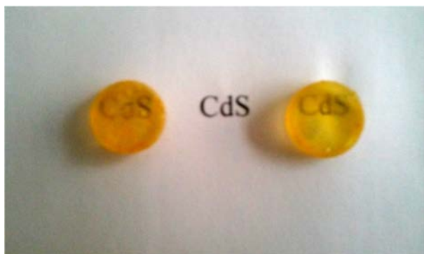
Fig. 3. Samples of structured poly(AcAm-AA) hydrogels filled with CdS nanoparticles ( \text{Cd}(\text{Ac})_2 = 25\% (left), 10% (right))
