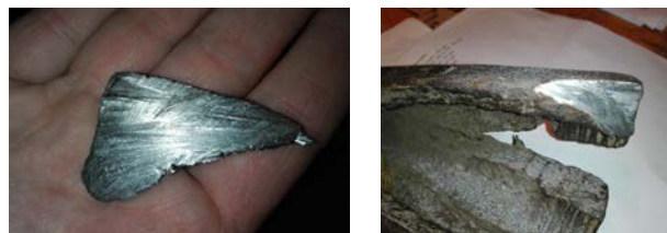
Picture 1. Specimen selection for microstructural analysis: a – blank for the specimen; b – destructed breeching part of the destroyed cannon
