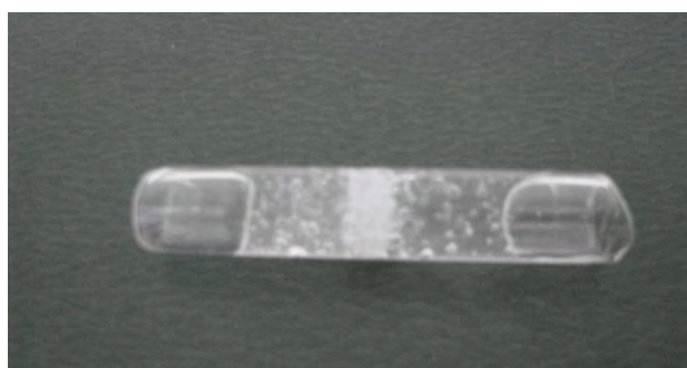
Fig. 3. Obtaining of the particles of hydroxyapatite in hydrogel
