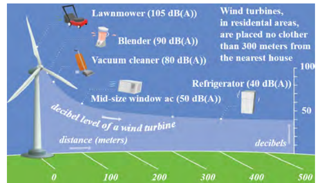
Fig. 1. The dependence of noise level on the distance between wind turbine and research object
