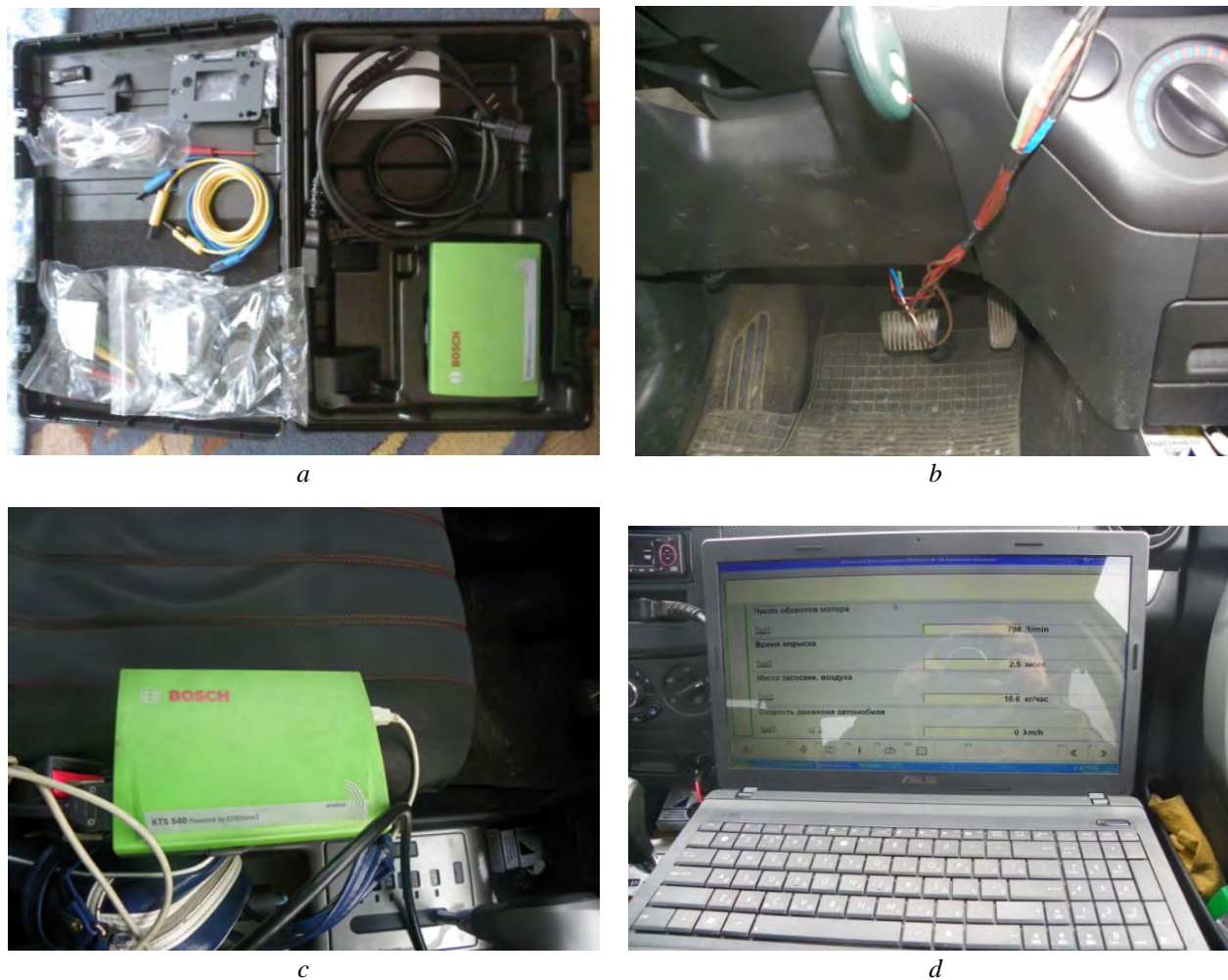
Fig. 2. The general view of the used equipment: a – complex Bosch KTS 540; b – connection of equipment to the diagnostic plug (connector) OBD-II of the motor vehicle; c – auto scanner Bosch KTS 540 in the cabin of the motor vehicle; d – display of the laptop with the installed software
