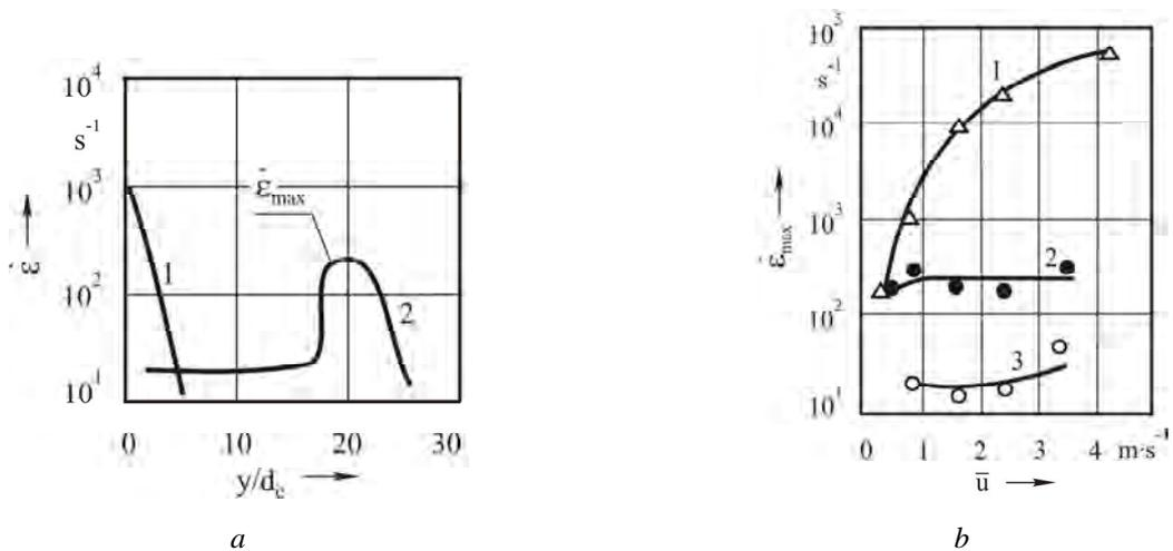
**Fig. 5.** *a* – velocity gradient distribution along the flow axis at  $\bar{u} = 0.8 \text{ m} \cdot \text{s}^{-1}$  for water (1) and 0.05 % PEO solution (2). Measurements were performed with the capillary I; *b* – dependence of the maximal longitudinal velocity gradient on the average flow rate for water (1) and 0.05 % PEO solution (2) and in the vortex for 0.05 % PEO solution (3)
