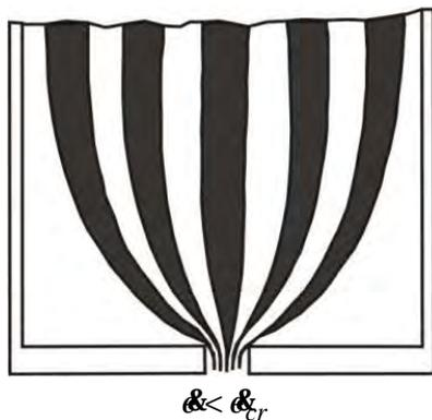
**Fig. 1.** Picture of flow in the inlet area of a capillary when injecting PEO solution into water during precritical mode of outflow
