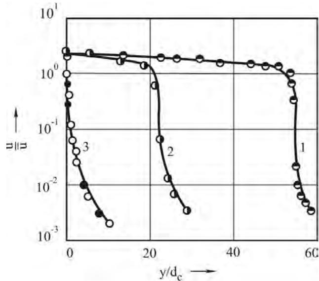
**Fig. 4.** Velocity distribution for the polymer solution along the flow axis:  $M_h = 4 \cdot 10^6$ , flow through the capillary I at the average flow rate  $\bar{u} = 2.5 \text{ m} \cdot \text{s}^{-1}$  (1), flow through the capillary II at  $\bar{u} = 0.8 \text{ m} \cdot \text{s}^{-1}$  (2) and through the capillary II at  $\bar{u} = 0.5 \text{ m} \cdot \text{s}^{-1}$  (3), filled circles represent the data for water when  $\bar{u} = 0.8 \text{ m} \cdot \text{s}^{-1}$
