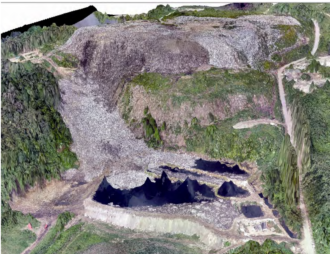
Fig. 5. Cloud points with imposition of orthophotoplan of Lviv landfill (June 2016)
