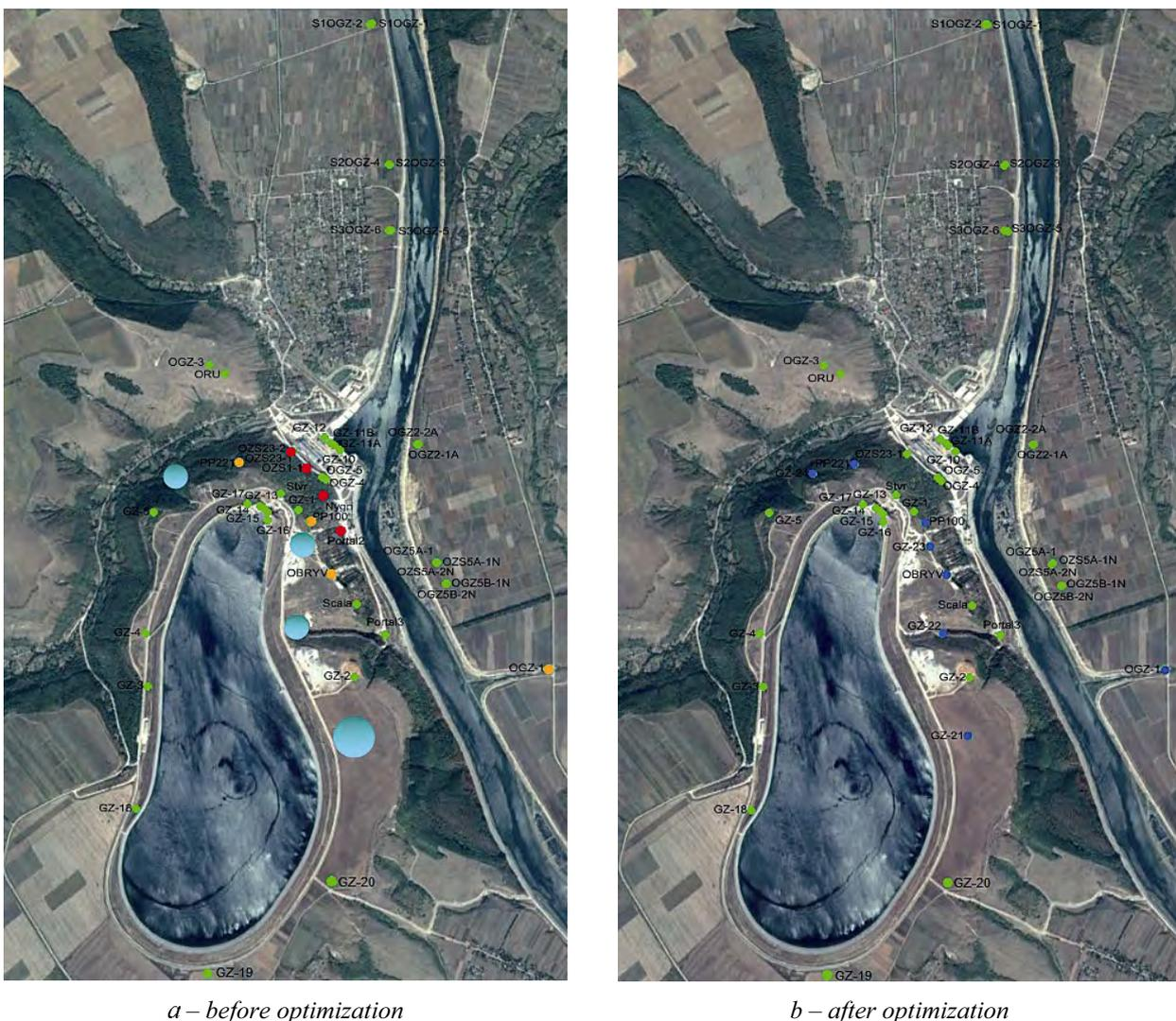
Fig. 3. Scheme of points of the reference Dnister PSPP based GNSS network
