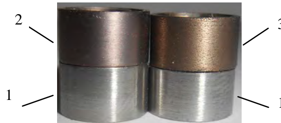
Fig. 8. The general view surface of the Zr-1 %Nb tubes after processing by the modes: 1 – P0, 2 – P4, 3 – P7
