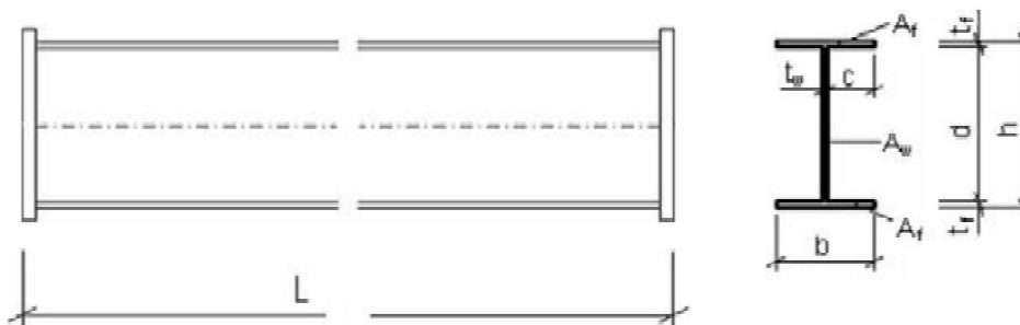
Fig. 1. Scheme of testing models/members
