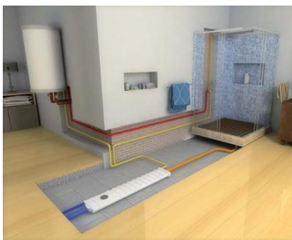
Fig. 4. Preheat of cold water combined with domestic hot water tank [3]
